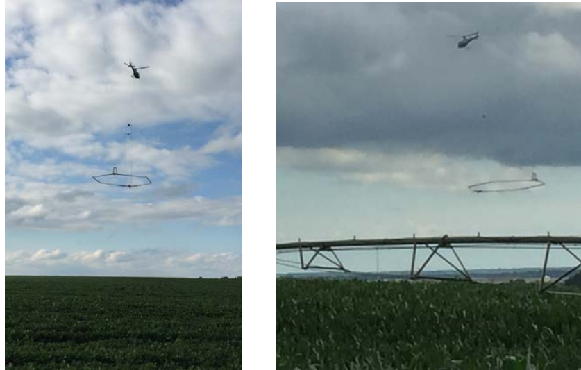
Figure 2-4: Photos of the SkyTEM304M/312 system in suspension beneath the helicopter.
